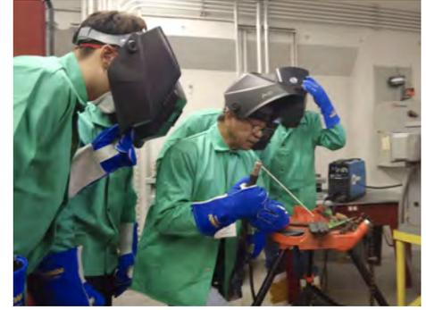
BM Val Ceria demonstrating a lap joint on two pieces of steel plates.
